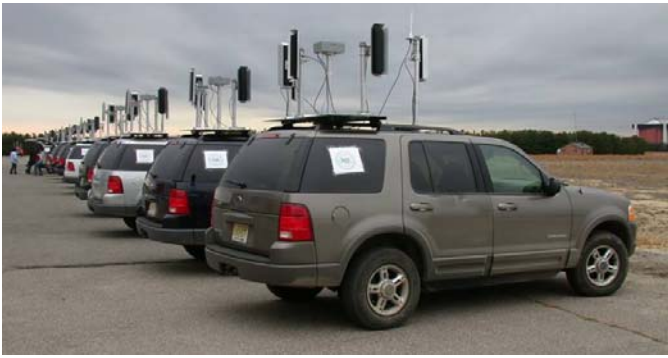
Fig. 3. Row of demo 1 vehicles. Mounted on top of each vehicle are four directional antennas, an omni antenna, and a mast holding the GPS device away from the vehicle.
